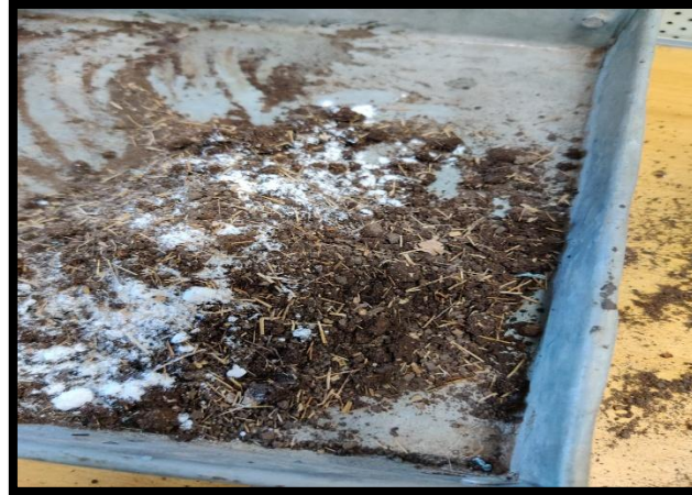
[Fig.4.8: Mixing of lime, bamboo fiber and black cotton soil]
