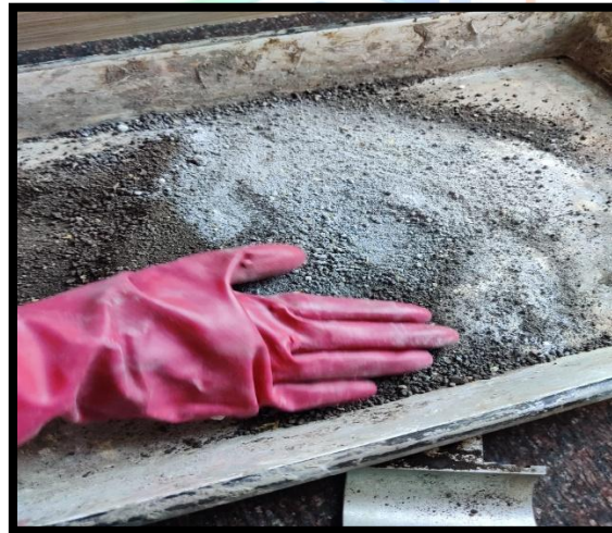
[Fig.4.6: Mixing lime with black cotton soil]
