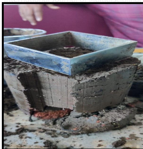
[Fig.4.4: Collect Undisturbed sample by using core cutter]
