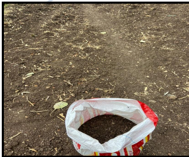
[Fig.4.1: Black cotton soil was acquired from the site at Achalpur, Amravati]
