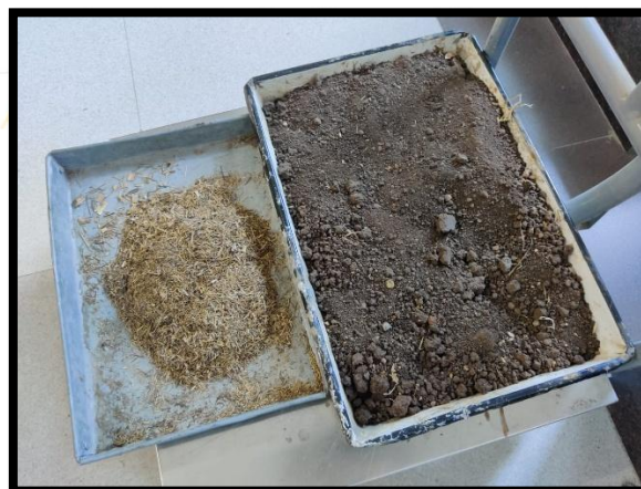
[Fig.4.7: Mixing bamboo fiber with black cotton soil]
