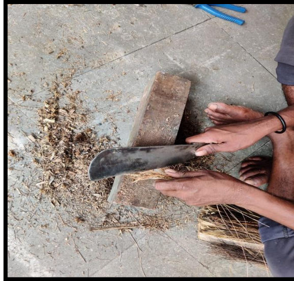
[Fig.4.5: Bamboo fiber cuts into grain size]
