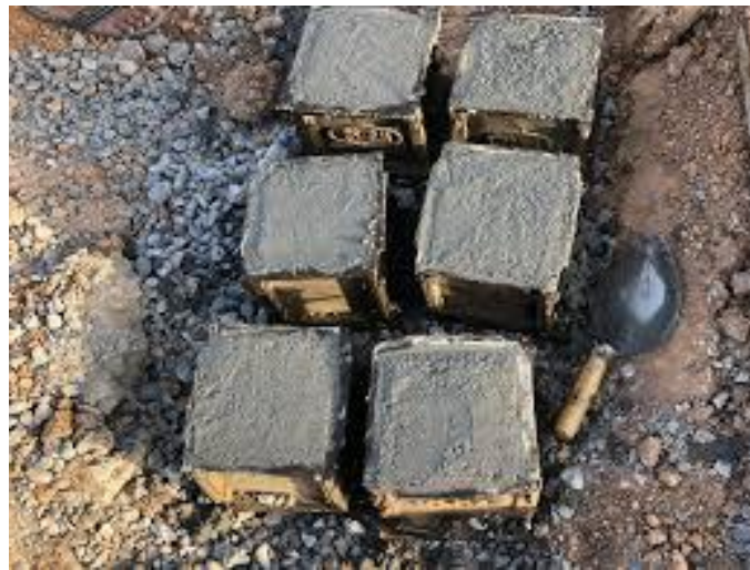
Fig 2.1: Casting of Concrete Cubes
