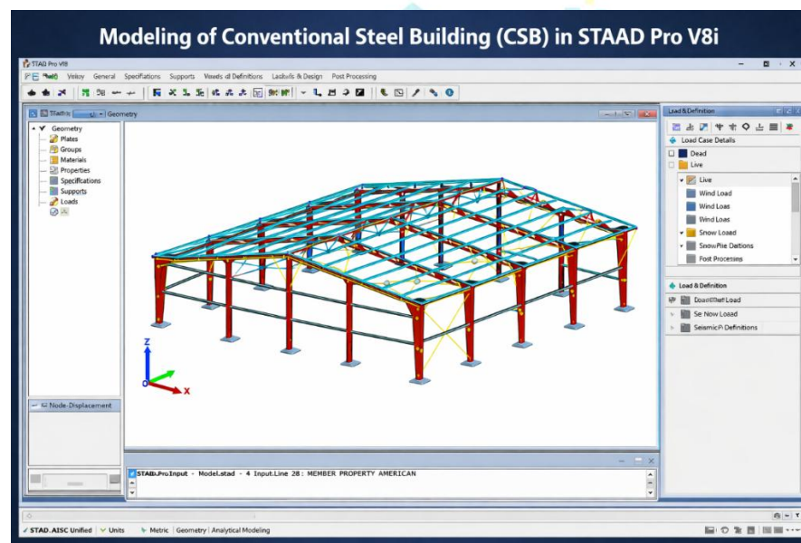
Figure 2.2: Software Modeling by using STAAD Pro V8i of PEB Structure
