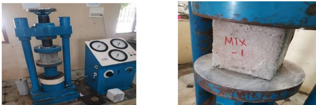
Figure 3.7: Compressive Strength Test
