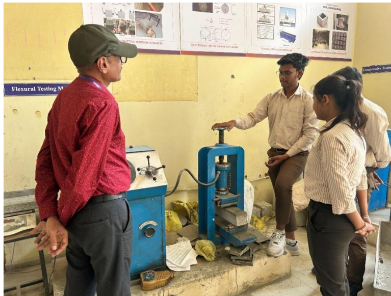
Figure 4.3: Flexural Strength Testing of Geopolymer Concrete Specimen Using Universal Testing Machine in Laboratory
