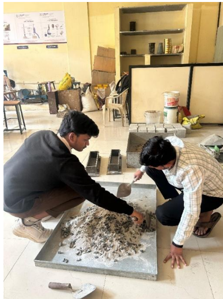
Figure 4.1: Manual Mixing of Geopolymer Concrete Incorporating Glass Powder in Laboratory Setup
