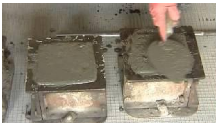
Figure 3.2: Casting of Cubes
