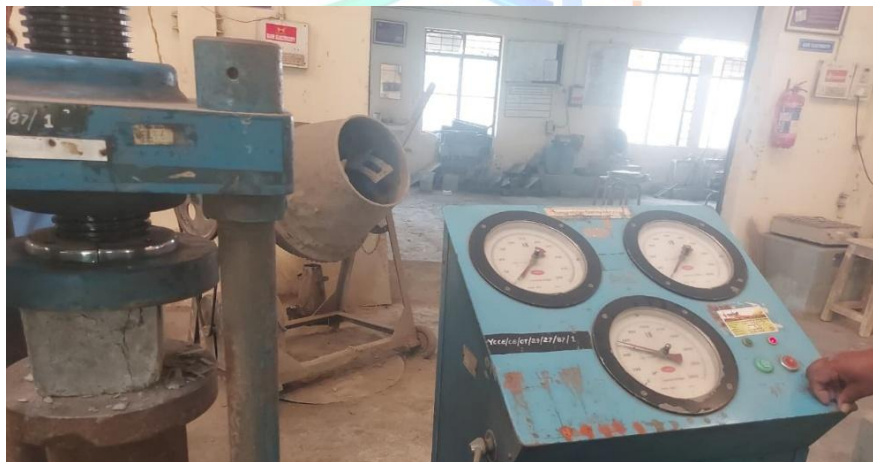
Figure 3.4: Compressive Strength Test
