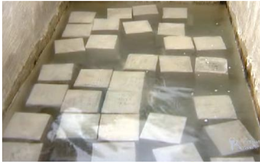
Figure 3.3: Curing of Cubes
