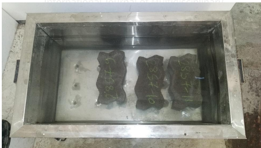
Figure 3.5: Water Absorption Test on Paver Blocks
