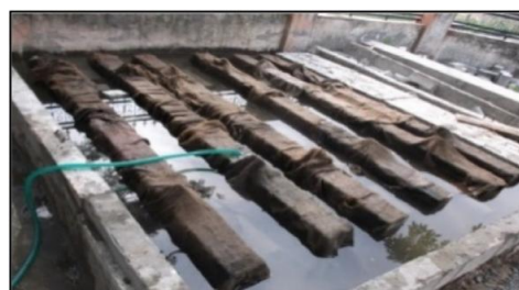
6(g) Test Beams Under Curing
