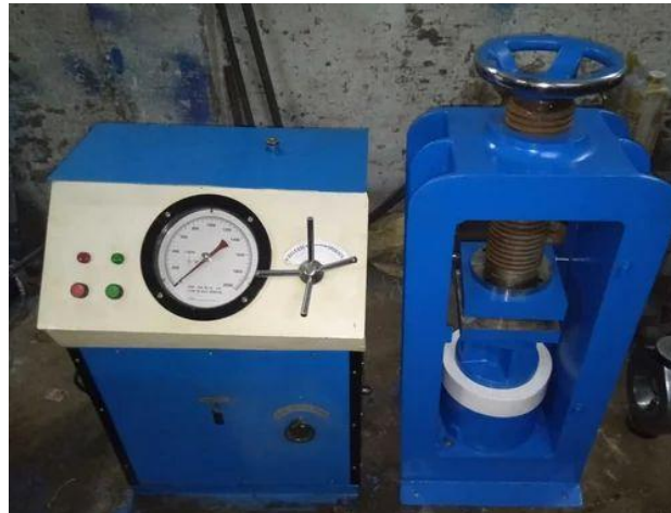
Figure 3.4: Compressive Strength Testing Using Compression Testing Machine
